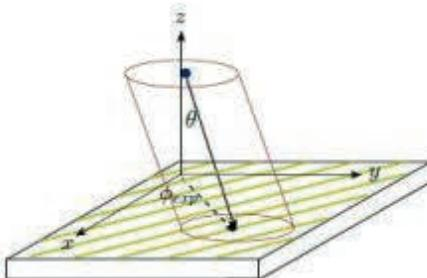
FIG. 1: A sketch showing the Monte Carlo modeling set-up for an ion-beam sputtering. As described in the text, an ion beam trajectory makes an angle  $\theta$  with the axes  $z$ , and the projection of the ion-beam direction on the  $x-y$  plane, makes an angle of  $\phi_{exp}$  relative to the  $x$  axis. Anisotropic direction is perpendicular to the  $x-y$  projection of the ion-beam.
