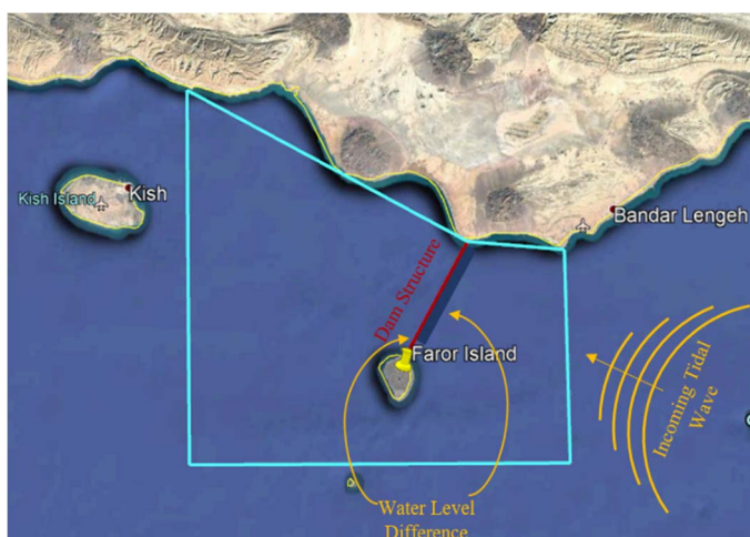
Fig. 1. Dynamic tidal power concept for the Faror island 2 .
