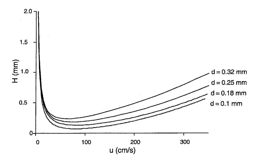
The values of  $H_{min}$  decrease, and the values of  $u_{opt}$  increase with decreasing column radius, and substantially faster separations can be obtained with the microbore (0.1-mm-i.d.) column.
