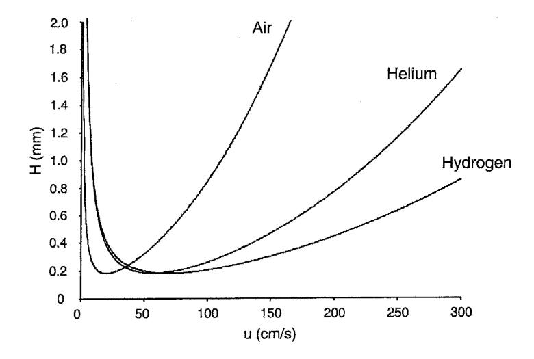
Note that the slope is inversely proportional to *jDG*. This explains why efficiency with helium as carrier gas decreases more rapidly with increasing *u* than with hydrogen. Thus, hydrogen become progressively more useful as a carrier gas for HSGC as the gas velocity increases. Air and nitrogen are particularly poor for HSGC, since  $u_{opt}$  is low and significant departure from u<sub>opt</sub> results in a large loss in efficiency.
