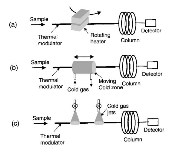
If a segment of a coated gas chromatographic column is operated at a lower temperature than the oven, or if the stationary phase film is thicker in that portion of the column, the increased retention factors for mixture components in the segment result in reduced migration velocities, and thus sample accumulation occurs in the segment.
