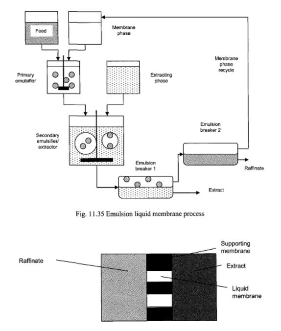
Fig. 11.36 Supported liquid membrane
