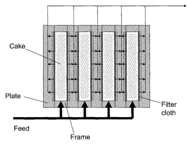
Operation of plate and frame filter press
