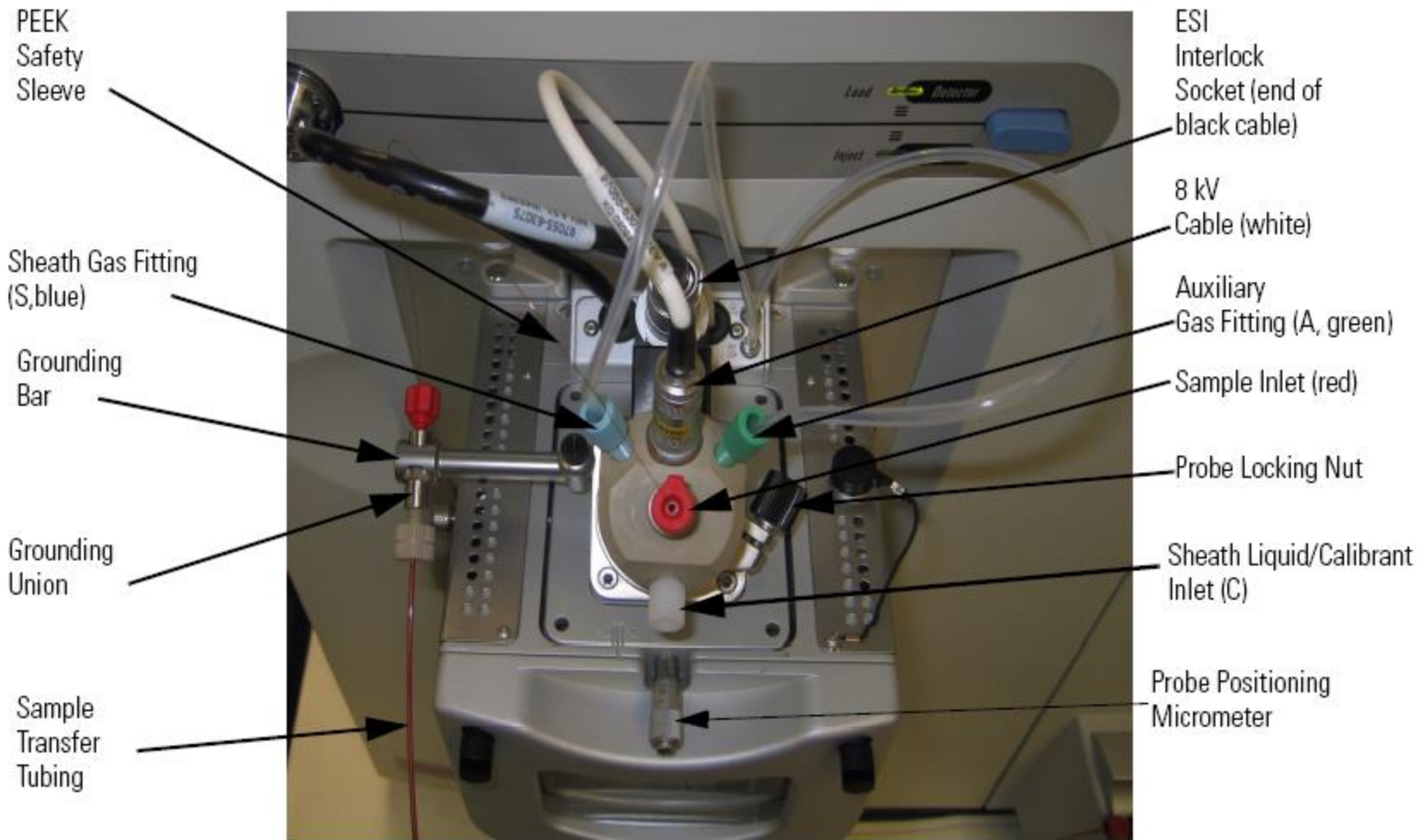
Figure 5. Ion Max ion source housing with ESI probe installed
