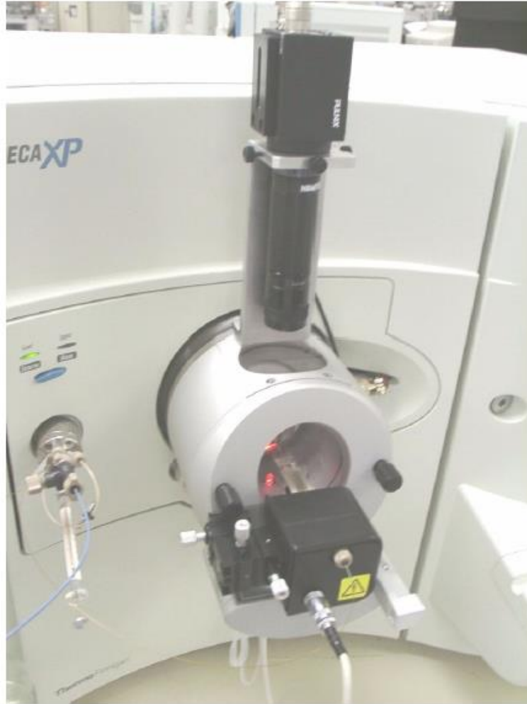
Figure 3-3. Camera mounted on the Finnigan LCQ Series MS detector
