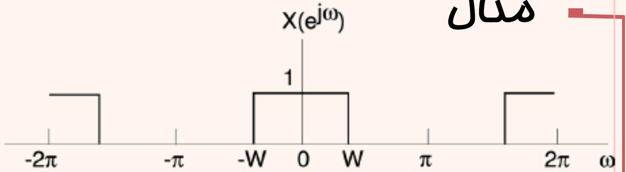
$$x[n] = \frac{1}{2\pi} \int_{-2\pi}^{2\pi} X(e^{j\omega}) e^{jn\omega} d\omega$$
