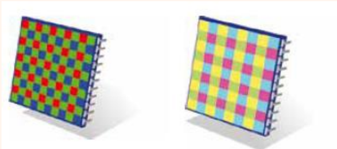
Bayer array color filter (left) and CMYG color filter array (right)
