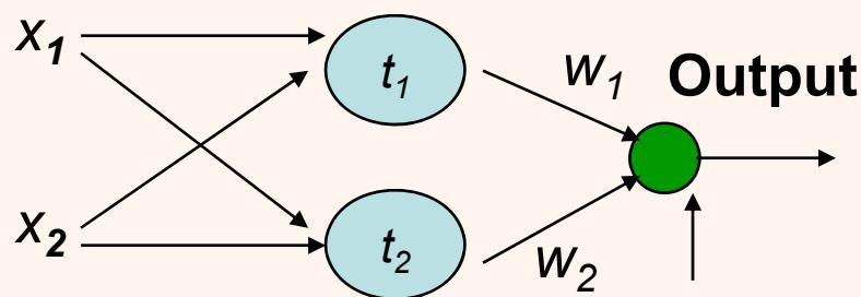
$$\mathbf{W} = (\Phi^T \Phi)^{-1} \Phi^T \mathbf{D} = \begin{bmatrix} -2.5 \\ -2.5 \\ 2.8 \end{bmatrix}$$
